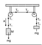
$$- mg + Mg + (T_3 - T_1) = Ma + ma$$
